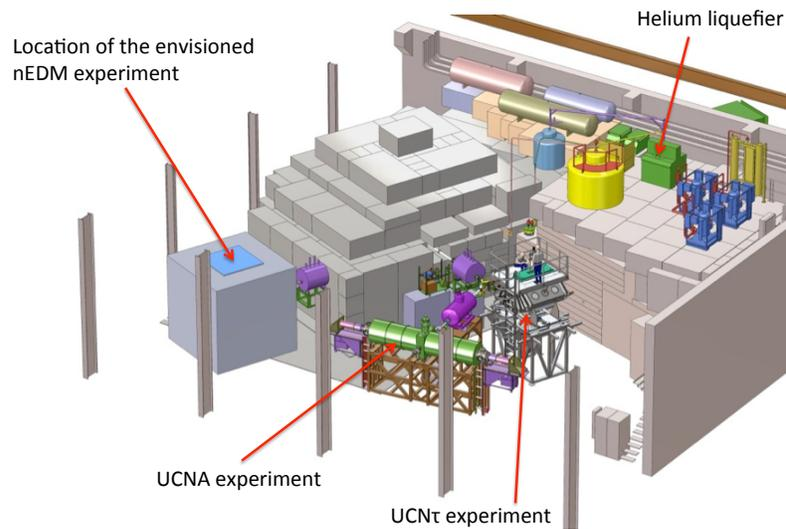
FIG. 1: Layout of the LANL UCN experimental area with the envisioned new nEDM experiment
