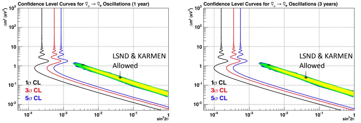
FIG. 3: The OscSNS sensitivity curves for the simulated sensitivity to  $\bar{\nu}_\mu \rightarrow \bar{\nu}_e$  oscillations after two (left) and six (right) *calendar* years of operation, assuming a 50% beam on-time (one and three years of running at 100% beam-on). Note that it has more than 5 $\sigma$  sensitivity to the LSND result in 2 years.
