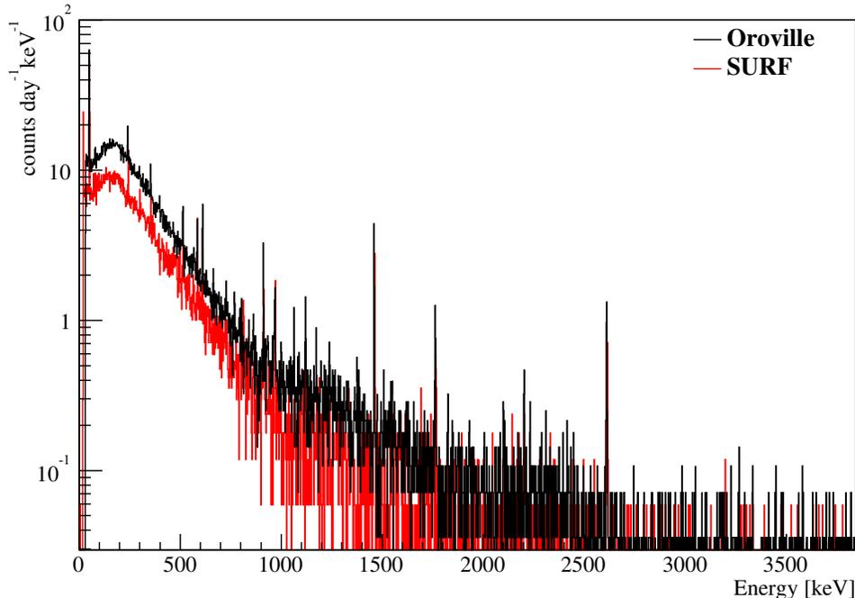
FIG. 2: Comparison of shielded ( $\text{N}_2$  purged) backgrounds at Oroville and SURF. The backgrounds at SURF are approximately 30% lower than that at Oroville, due to some minor improvements in the shield configuration.
